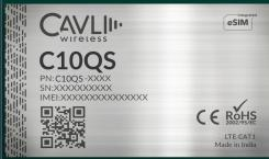
LTE CAT 1 Module compliant with 3GPP release 10
